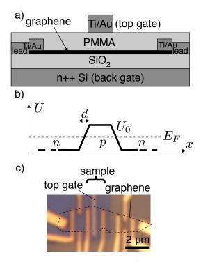
FIG. 18 *n-p-n* junction in graphene: a) cross-sectional view of the device. b) electrostatic potential profile U(x) along the cross-section of a). The combination of a positive voltage on the back gate and a negative voltage on the top gate produces a central *p*-doped region flanked by two *n*-doped regions. c) Optical image of the device. The barely visible graphene flake is outlined with a dashed line and the dielectric layer of PMMA appears as a blue shadow. (Huard et al., 2007)
